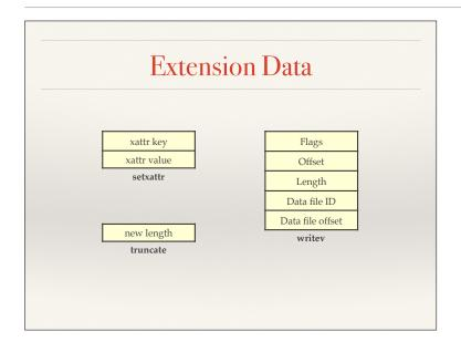
Extension data can take many forms, depending on the type of the user I/O request. These are just examples. Note that the *writev* example has two offsets - one within the actual file and one within the journal data file. The second offset, along with the data file ID, defines where the data landed <u>within the journal</u> before being destaged to the main file store.
