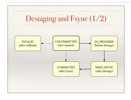
The life cycle of a request is shown above. As part of the higher-level protocol, the first NEW\_REQUEST entry for a request puts it in UNCOMMITTED state. At our local discretion we destage, adding STATE\_CHANGE events to IN\_PROGRESS and NEED\_FSYNC around the actual main-store operation. Finally, when a user's fsync request comes in (or at our local discretion) we issue a local fsync and add a final STATE\_CHANGE(COMMITTED) event. (continued)
