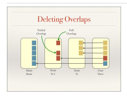
Because data which is "covered" by a write in a later term is no longer useful even for reconciliation, it shouldn't be included in filters (described later) either. Special OVERLAPPED events, similar to ROLLBACK events, are added to reflect such changes. Note that for a partial overlap this event might truncate or split the original event instead of quashing it entirely. These optimizations can all be done locally on each replica.
