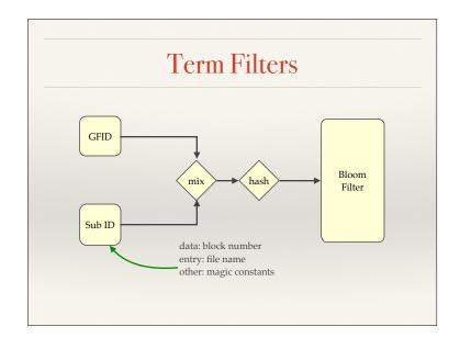
We maintain and store a Bloom filter for each term, to enable efficient determination of whether the term contains anything at all relevant to a subsequent read (or reconciliation). Each data block, directory entry, or metadata field is treated as a separate entity for filter purposes, even if a single request affects multiple entities. For each entity, we calculate a hash and use that to populate the term's Bloom filter.
