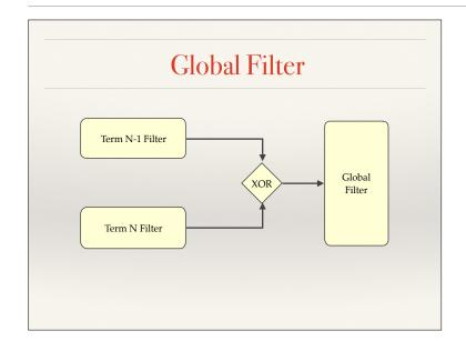
We also maintain a global filter, to determine quickly whether <u>any</u> term still contains relevant data for a read or reconciliation. To avoid "filter pollution" the global filter is kept at a coarser granularity than per-term filters by using only GFIDs without futher refinement by sub-ID (e.g. block number). We do calculate and store GFID-only filters for each term, but only to enable (re)calculation of the the global filter.
