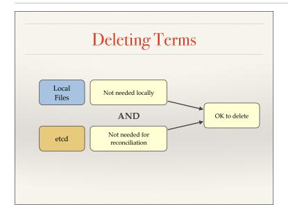
A term can only be deleted when two conditions are met - it's not needed locally (i.e. all data has been fully destaged and fsync'ed) and it's not needed for reconciliation. Therefore, we must check for eligibility whenever either of these conditions change.
