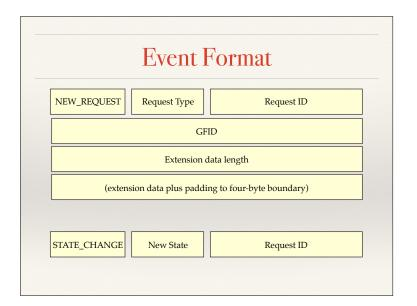
All entries in the event log start with a four-byte header, starting with an event type. The other contents of the header can vary depending on the event type. For the most common NEW\_EVENT and STATE\_CHANGE types, these contents include a request ID that is used to associate all related events with one another. In the special case of NEW\_REQUEST, extra information describing the request follows the header, and is described on the next slide.
